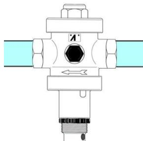
The pressure reducers EUROBRASS 146 don't get the effects, in their functioning, of gravity force; therefore they can be installed in the plant in any position:
